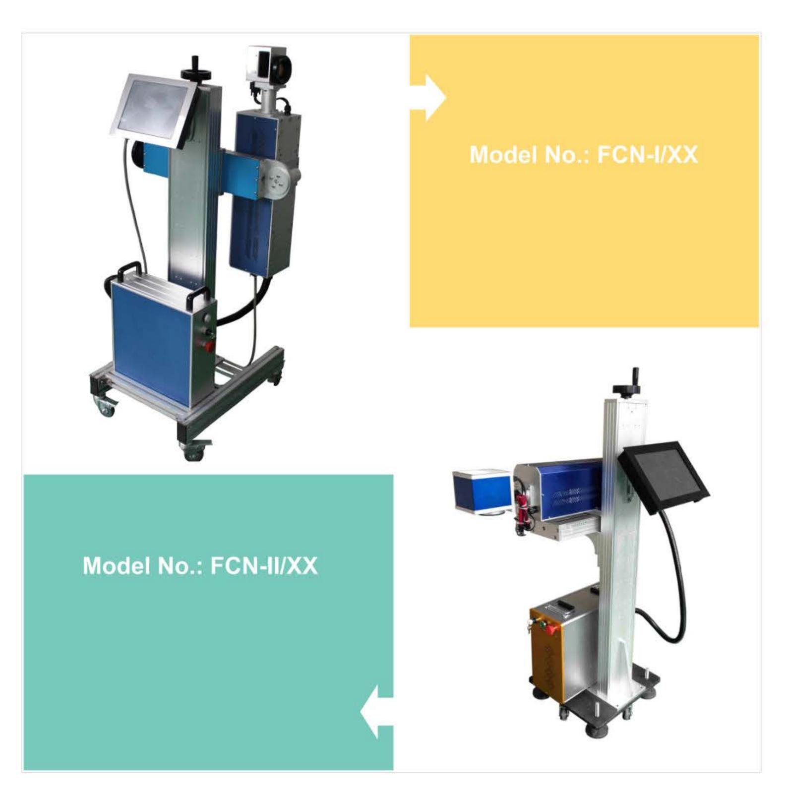
Combine laser technology with production line, it can mark on fast moving products. It is mainly used in marking characters, figures, batch numbers, production dates, validity, LOGO, real time clock information and anti-counterfeiting, especially the pharmaceutical industries GMP and food industries HACCP.
